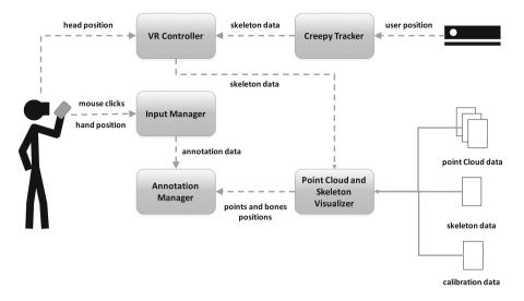
Fig. 1. Virtual Reality Annotator modular architect diagram
